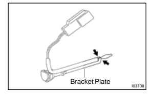
(c) Release the 2 claw and remove the thermistor from the bracket plate.
